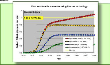
The figure above shows several scenarios that assume biochar production from waste biomass only, which is a small fraction of Earth's annual net primary production (NPP). Counting only the impacts of biochar burial in soil, and without considering the displacement of energy from fossil fuels, we can conservatively offset one quarter of a gigaton of carbon annually by 2030.
