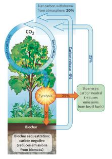
**Biochar can sequester or store carbon** in the soil for hundreds and even thousands of years. Biochar also improves soil fertility, stimulating plant growth, which then consumes more CO<sub>2</sub> in a feedback effect. And the energy generated as part of biochar production can displace carbon-positive energy from fossil fuels.
