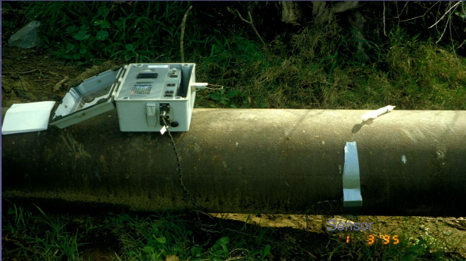
pipe cross-sectional area X water velocity = Flow rate
