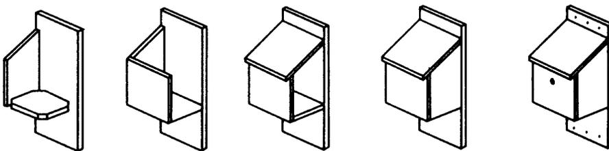
Figure 2. Assembly sequence.
