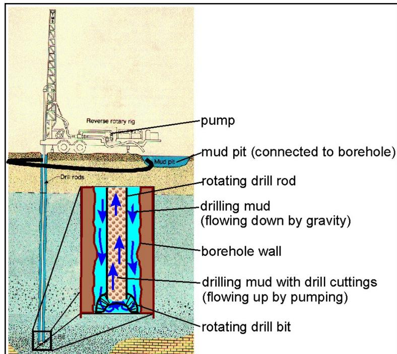
Figure 23. Reverse-rotary drilling method.
