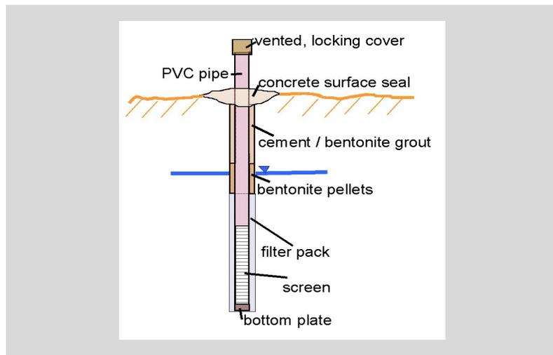
Figure 21. Principal components of a production or monitoring well in California.
