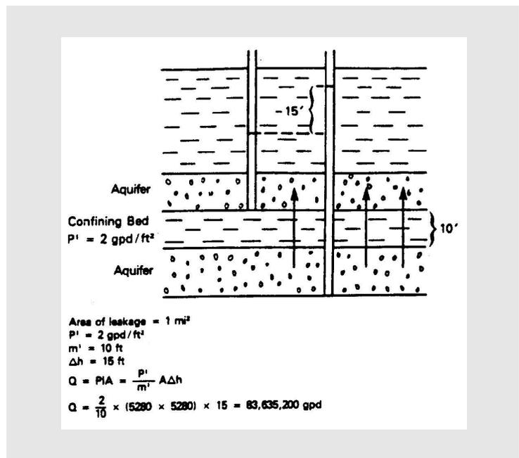
Figure 4: Using Darcy's law to calculate the quantity of leakage from one aquifer to another. (From EPA, 1994, Figure 4-9)
