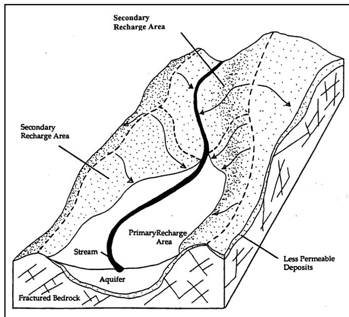
Figure 14: Illustration of the concept of recharge area (primary recharge area) and source area (secondary recharge area). (From California DWSAP, Figure 6-2)
