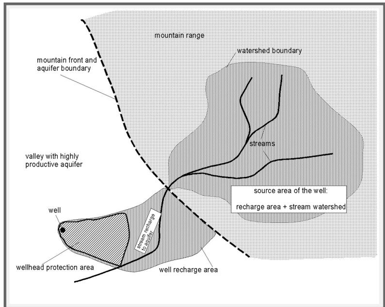
Figure 1: Conceptual illustration showing the relationship of wellhead protection area, recharge area, and source area of a well.
