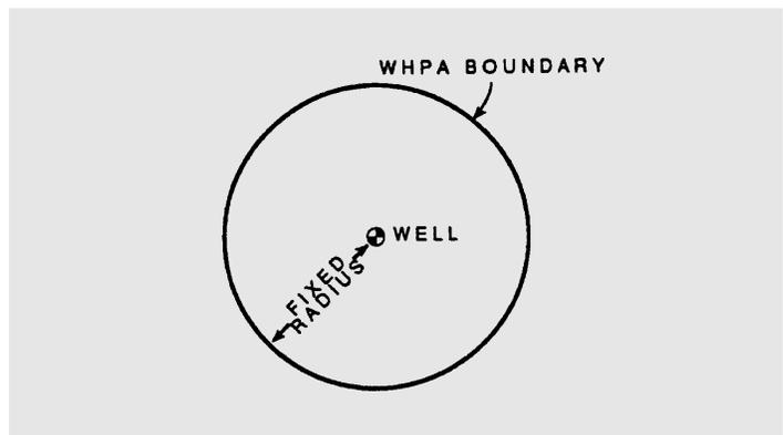
Figure 2: Delineation of wellhead protection area by fixed radius method. (From EPA, 1994, Figure 4-4)
