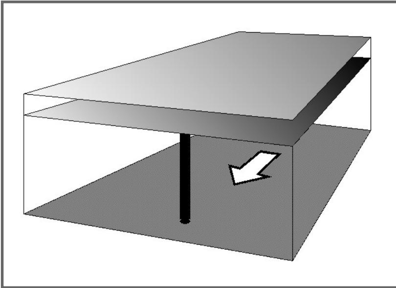
Figure 8: Geometric or analytical methods work best where the relevant extent of the aquifer can be described by simple geometry (uniform aquifer thickness, permeability, and groundwater flow direction).
