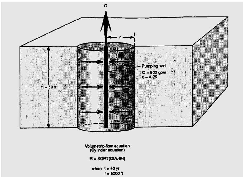
Figure 3: Delineation of wellhead protection area by cylinder method. (From EPA, 1994, Figure 4-4)
