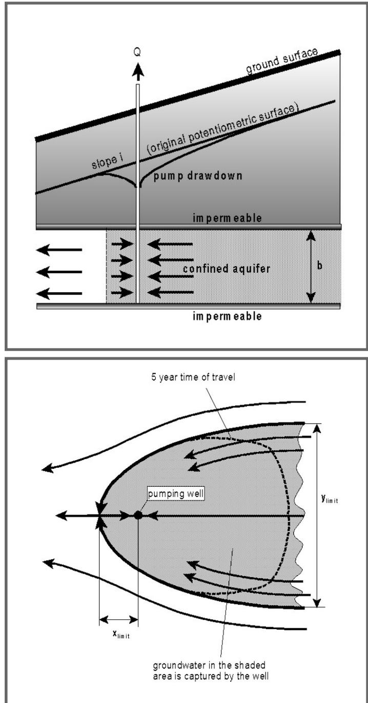
Figure 13: Flow to a well in a uniformly sloping potentiometric surface: (a) cross-section (upper), and (b) plan view (lower). (Modified from EPA, 1994, Figure 4-10)
