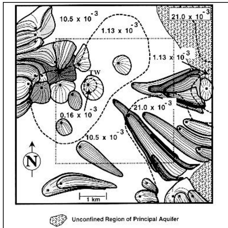
Figure 10: Fifteen-year TOT zones (shapes with flow lines) in a confined aquifer with a complex flow field. Contour lines delineate areas of varying hydraulic conductivities. (From Forster, C. B., T. E. Lachmar, D. S. Oliver, 1997)
