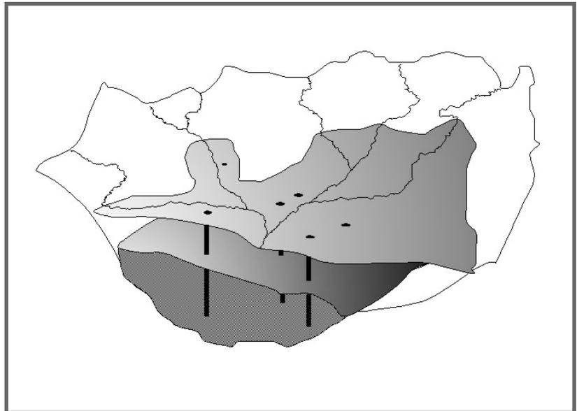
Figure 9: When the aquifer geometry is complex and multiple pumping wells are located near each other, numerical computer modeling may be the best tool for delineating groundwater protection zones.
