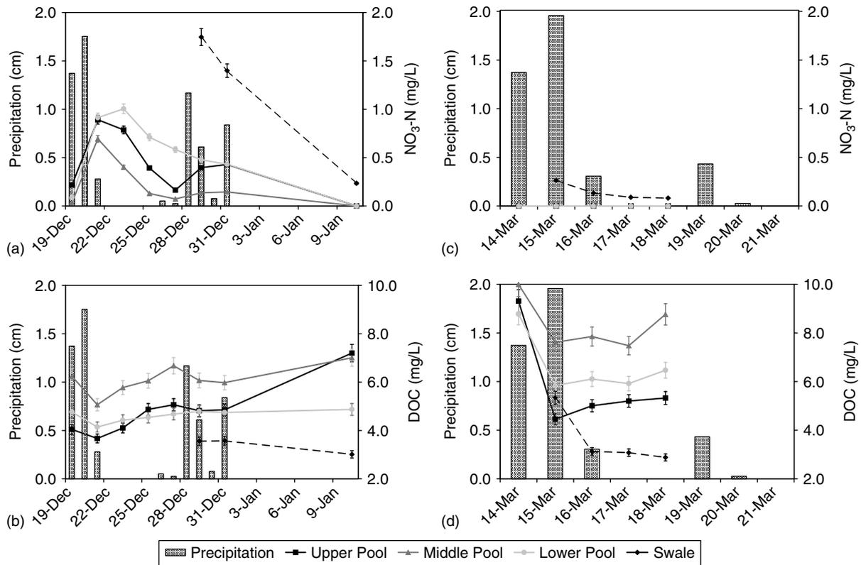
Figure 9. Daily precipitation and (a)  $\text{NO}_3\text{-N}$  and (b) DOC concentrations in vernal pool water during the early-season storm event, and daily precipitation and (c)  $\text{NO}_3\text{-N}$  and (d) DOC concentrations in vernal pool water during the late-season storm event
