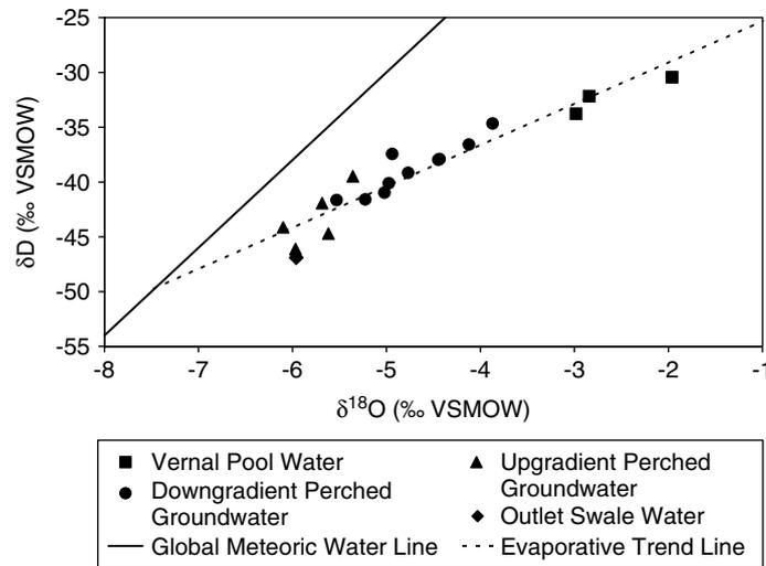
Figure 7. Scatterplot of  $\delta D$  and  $\delta^{18}O$  in vernal pool water (squares), upgradient perched groundwater (triangles), downgradient perched groundwater (circles), and outlet swale water (diamonds). The global meteoric water line (Craig, 1961) is the solid line and the evaporative trend line calculated via least-squares regression is the dashed line. Only surface water and perched groundwater samples collected between storms in early March 2003 are included
