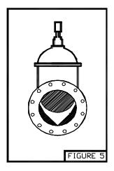
were not a significant controlling factor might be to install a VFD with a line bypass and a gate valve with a 90 degree 'V' shaped orifice.
