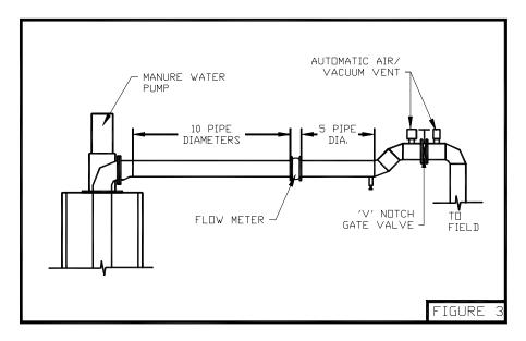
straight section to insure that the pipe is always full of water. An air vent is provided after the rise to insure that all air has been vented from the pipe. It is generally more challenging to design gravity irrigation metering runs due to the small head pressure sometimes available and the difficulty of insuring that the pipe is always full of liquid.
