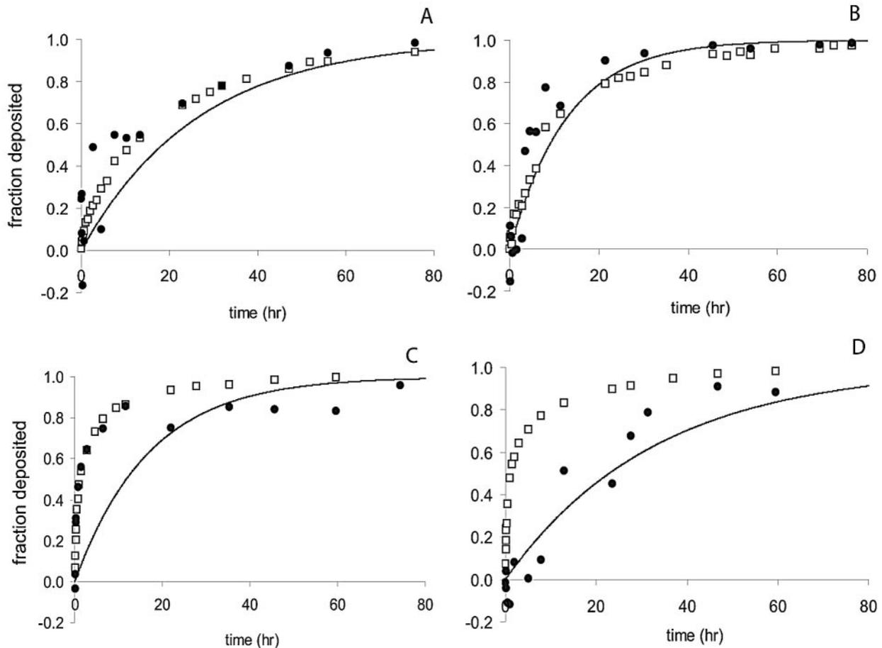
FIG. 3. The fraction of suspended sediments (open squares) and oocysts (dark circles) deposited in the sediment bed of the recirculating flume over time. The line represents the stream-subsurface exchange model prediction for the removal of oocysts in flume experiments with kaolinite particles (A), iron oxide particles (B), Des Plaines River sediments (C), and Salt Creek sediments (D).
