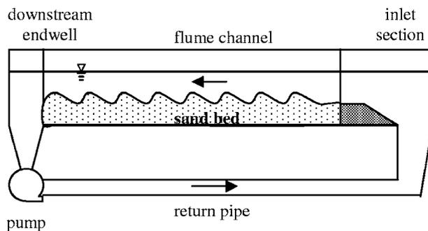
FIG. 1. Schematic diagram of the recirculating flume used for *C. parvum* oocyst deposition experiments.
