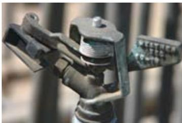
**Figure 1.** Close-up of an impact sprinkler head with the nozzle and orifice size ( $7/16$ ) stamped on the nozzle.
