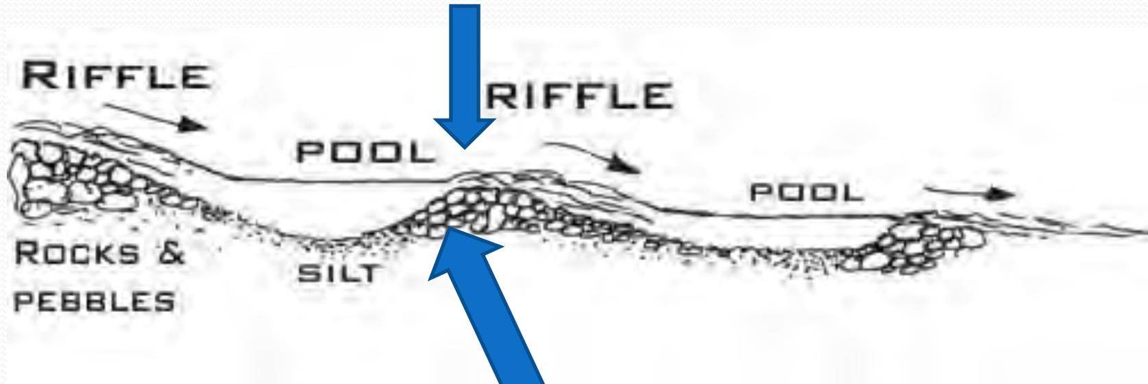
Measurements made upstream of crest, at distance 10% of pool length from crest
