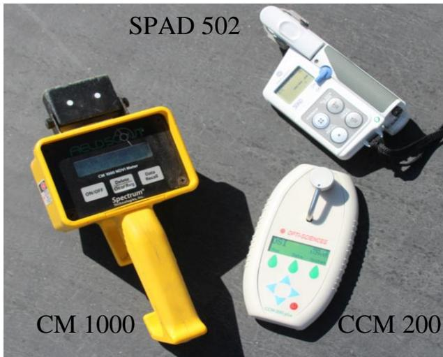
Very good correlations were observed between meter reading differences from the CCM 200 and SPAD instruments and nitrogen recommendation,  $R^2 > 0.89$  and  $0.90$ , respectively. CM 1000 measurements made early in the season were not well correlated because too much bare soil was sampled in the measurement area thereby making those measurements less reliable.
