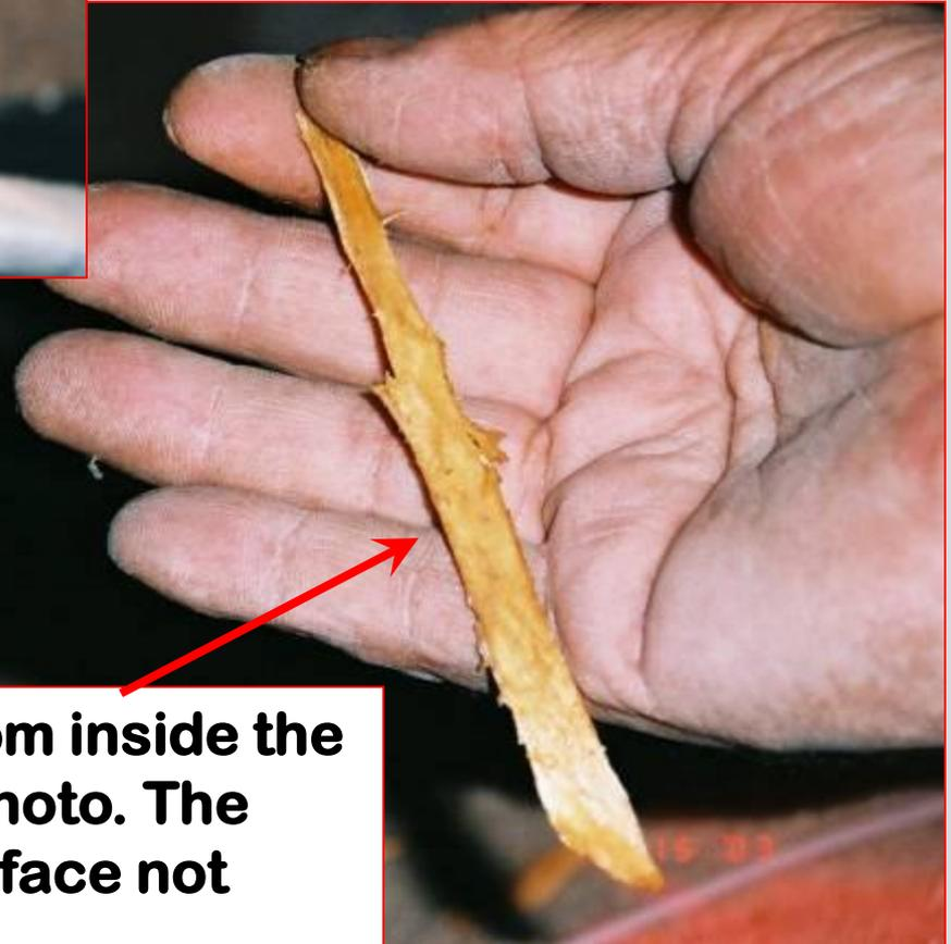
A fresh rhizomorph, taken from inside the girder shown in the top left photo. The girder was opened up on the face not visible in the above photo.
