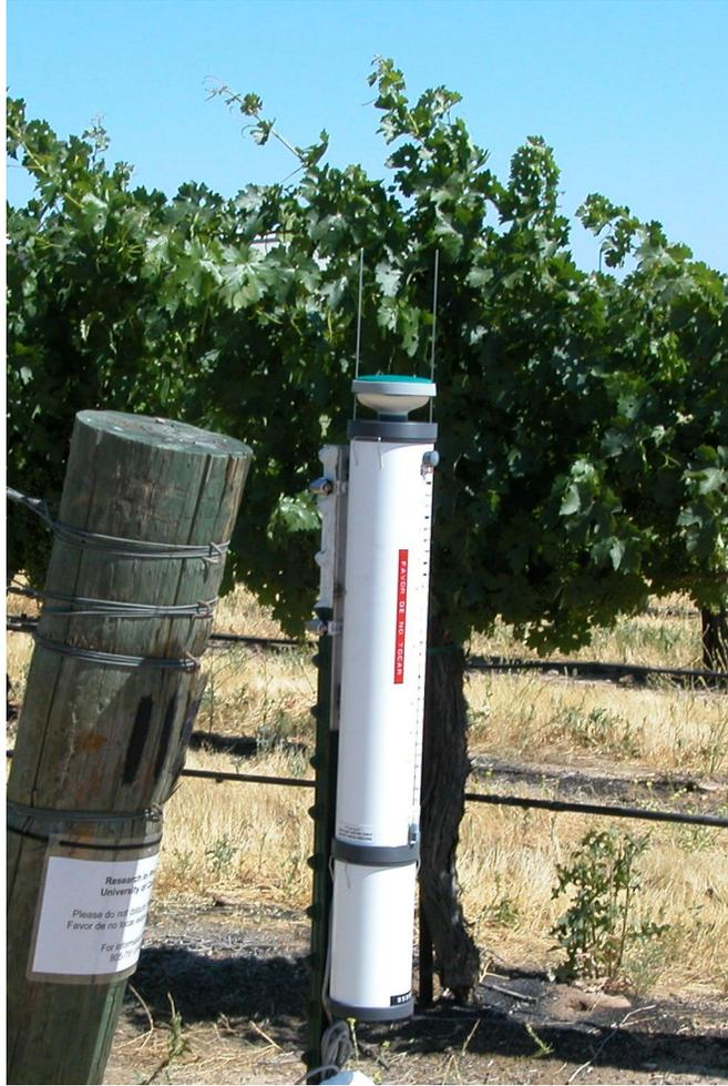
Figure 1. An atmometer installed on a steel fencepost at the end of a vineyard row.
