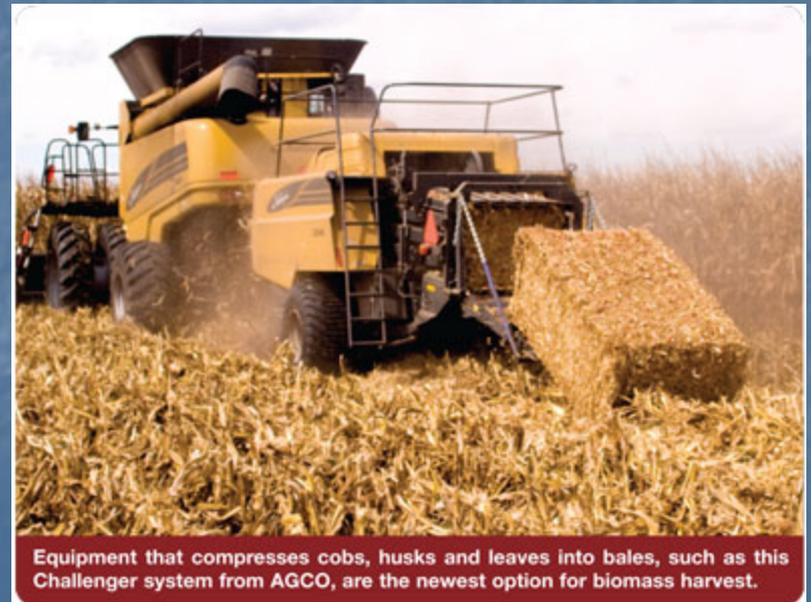
Equipment that compresses cobs, husks and leaves into bales, such as this Challenger system from AGCO, are the newest option for biomass harvest.
