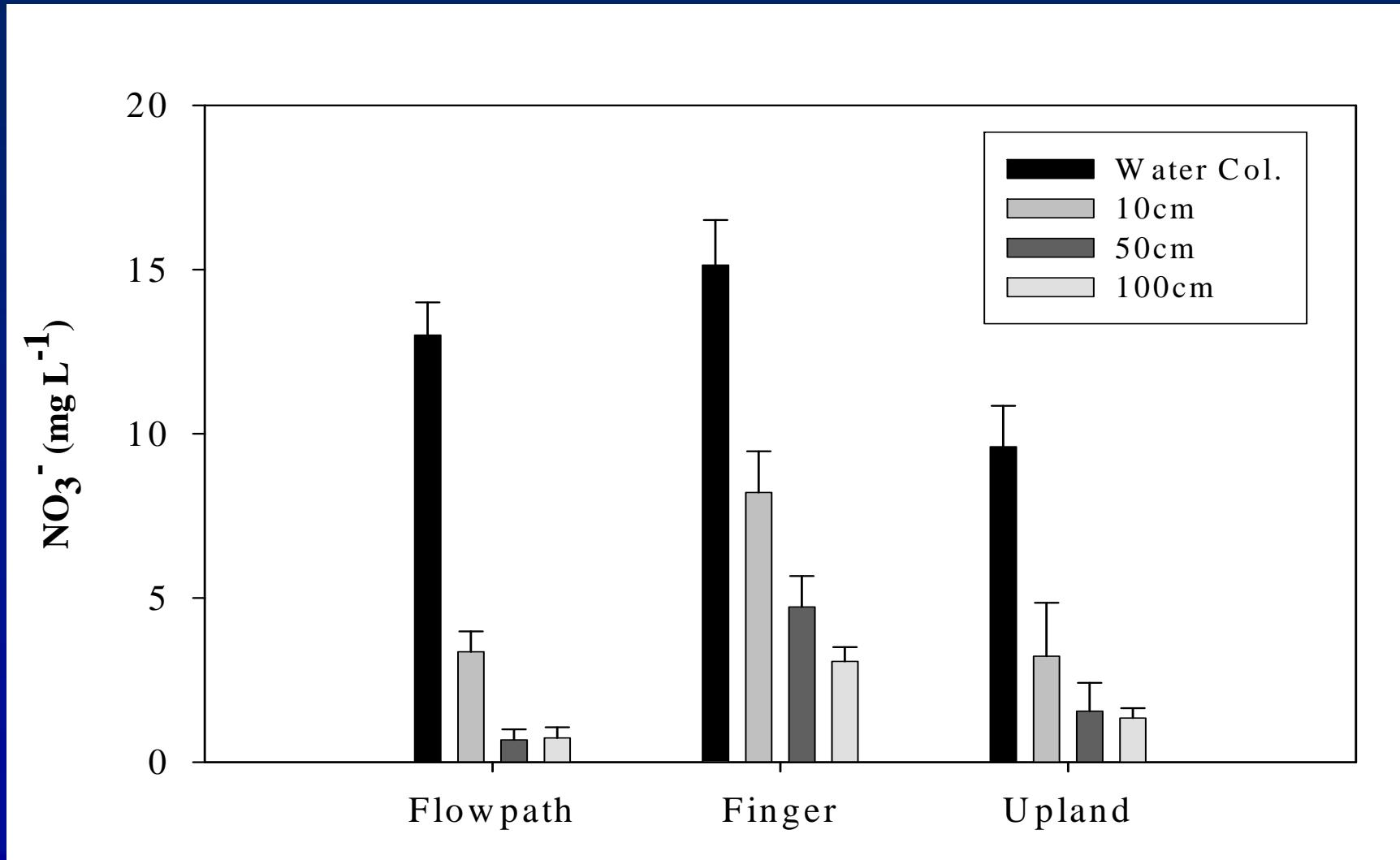
**Denitrification is the main mechanism for nitrate removal; occurs in soils where oxygen content is low (low redox potentials).**
