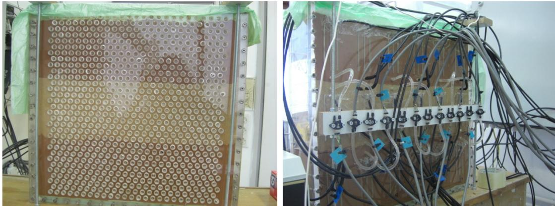
*Figure 1: images of Hele-Shaw cell. Sampling wall (left) and TDR/tensiometer/redox wall (right)*
