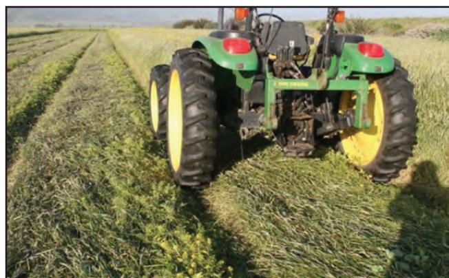
Figure 18: Terminating cover crops on beds using a roller crimper. (Eric Brennan)
