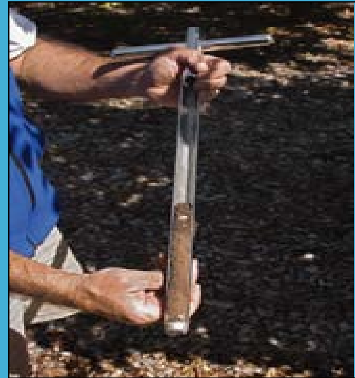
Soil sampling tube
