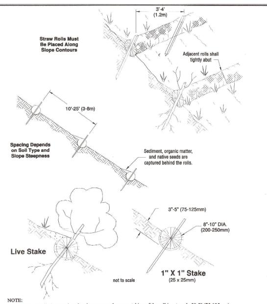
1. Straw roll installation requires the placement and secure staking of the roll in a trench, 3"-5" (75-125mm) deep, dug on contour. runoff must not be allowed to run under or around roll.
