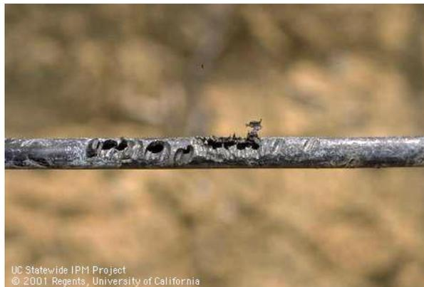
Holes chewed in a microsprinkler drip line by California ground squirrel, *Spermophilus beecheyi*.
