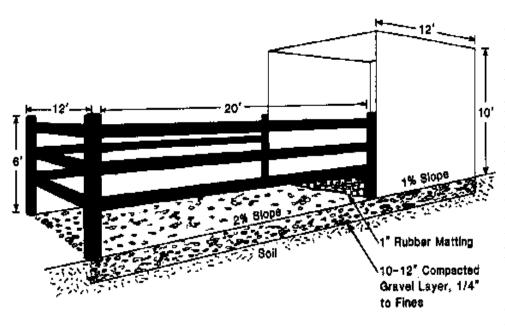
Figure 2 provides another example of a paddock (12 ft. wide by 20 ft. long) for a single horse. In this design the entire surface is prepared for adequate drainage. A 10" to 12" layer of pea gravel is covered with decomposed granite (DG) to serve as a cushion and help prevent foot sores and lameness. Under the shelter, the DG layer is covered with 1" rubber matting.
