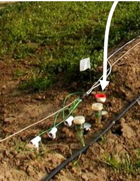
A device using low levels of radiation, the neutron probe, was developed in the 1960's for checking soil moisture. Used mostly by researchers and irrigation consultants, it is often the standard check for the accuracy of other instruments. Largest sample "volume" to estimate moisture.
