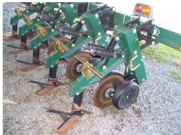
Figure 3. High residue cultivator
