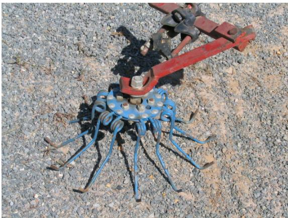
Figure 8. Flexible spider weeder
