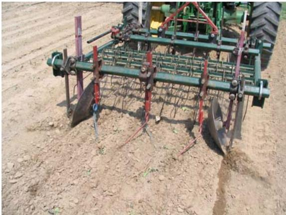
**Figure 5. Flex-tine weeder with torsion rods**
