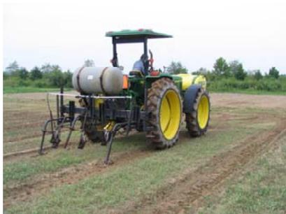
**Figure 7. Flame weeder on tractor**
