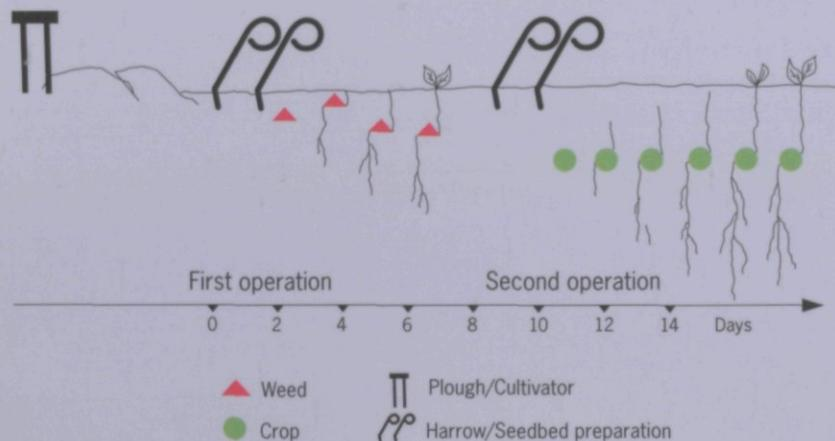
Harrowing during the period between sowing and the emergence of the shoots is feasible only when the germinating seeds of the crop are deeper than the harrow's cultivation depth.
