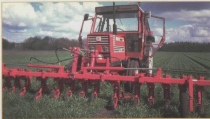
The hoes mounted on the toolbar can be either rigid blades or spring tines (vibrating hoe). A number of hoes can be fitted between two rows when the distance between the rows is 25 cm or more. The major benefit offered by this approach is the continually variable hoeing width. Together with the working width of the hoes between the crop rows, the soil cultivation achieved with the hoes is also of importance. The ideal hoeing depth is 1 to 2 cm.
