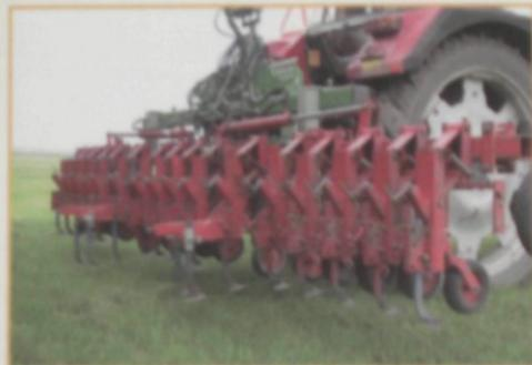
Hoe beam with parallelograms and hoe blades.
