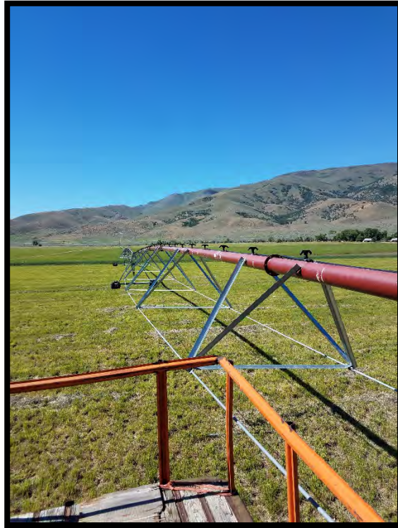
Double Goosenecks installed on the top of pipe, to double the number of drops. (The other pivot tested used triple goosenecks.
