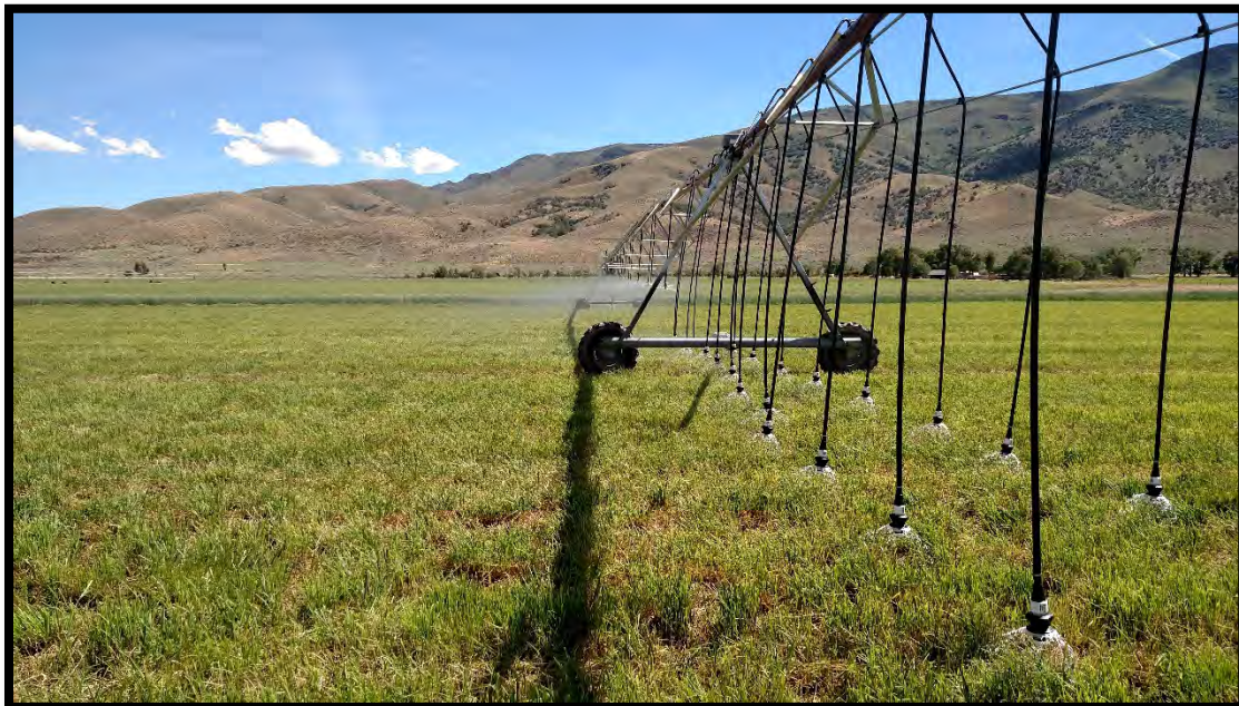
Photo of LESA system up front, bubbling water down, notice the wind blowing water from the standard sprinklers in the background.
