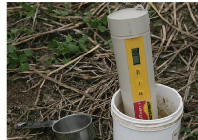
Soil pH can be measured with a pocket pH meter and used as an indicator of potential nutrient deficiencies.
