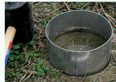
Water infiltration is measured using a ring infiltrometer; if soil is severely compacted, sit back and wait.
