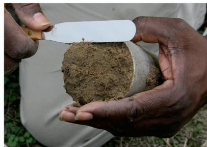
Higher bulk densities can indicate less pore space, less oxygen and increased resistance to root penetration.
