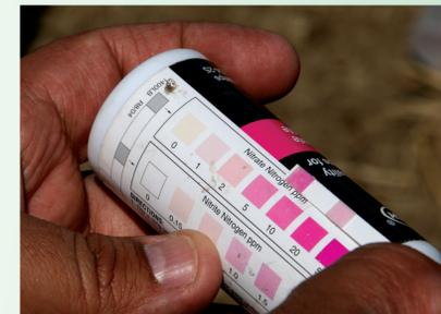
A nitrate test strip can be used to determine nitrate-nitrogen levels in the soil.
