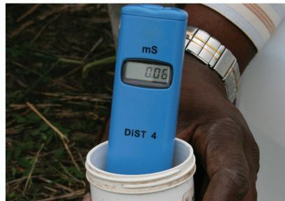
A pocket electrical conductivity meter is a quick method to measure salts in the soil solution.
