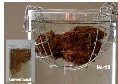
The Slake Test demonstrates a soil's ability to retain its structure and allow water to infiltrate into it.
