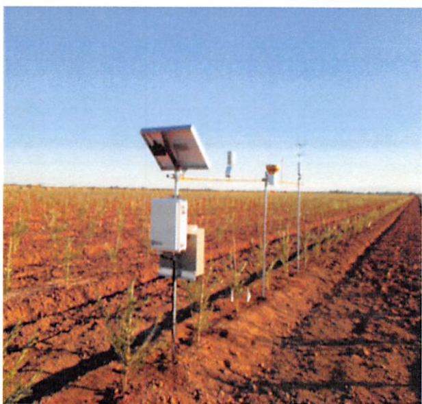
Figure 2. ET measurement equipment installed at a young olive orchard in the Imperial Valley
