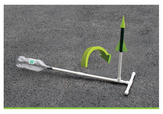
Step 3: Slide the rocket down the launch tube.
