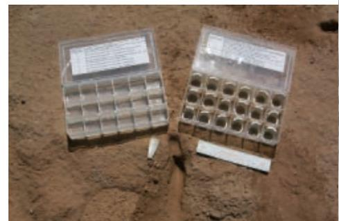
**Figure 5.** Complete soil stability kit with water and samples.
