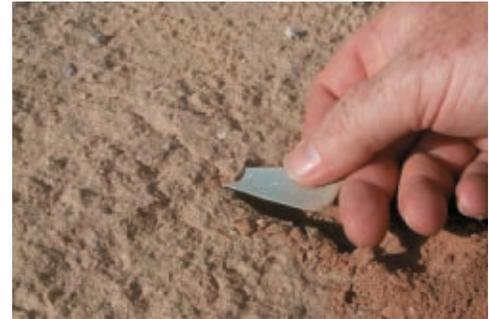
**Figure 2.** Collect surface sample.
