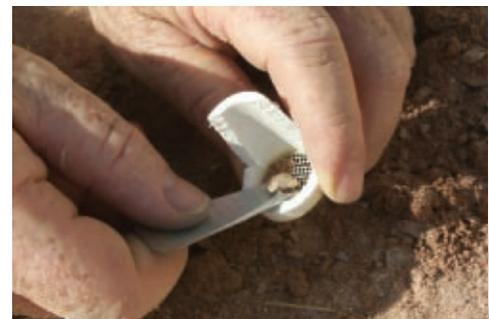
**Figure 4.** Place sample in sieve.
