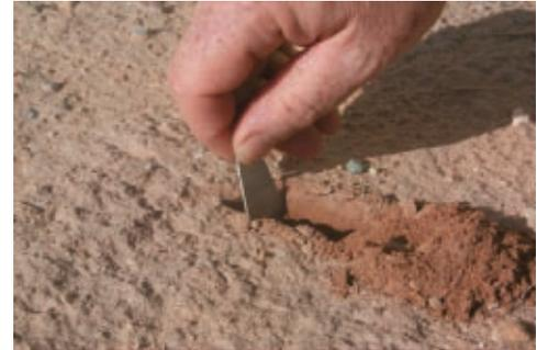
**Figure 1.** Excavate small trench.
