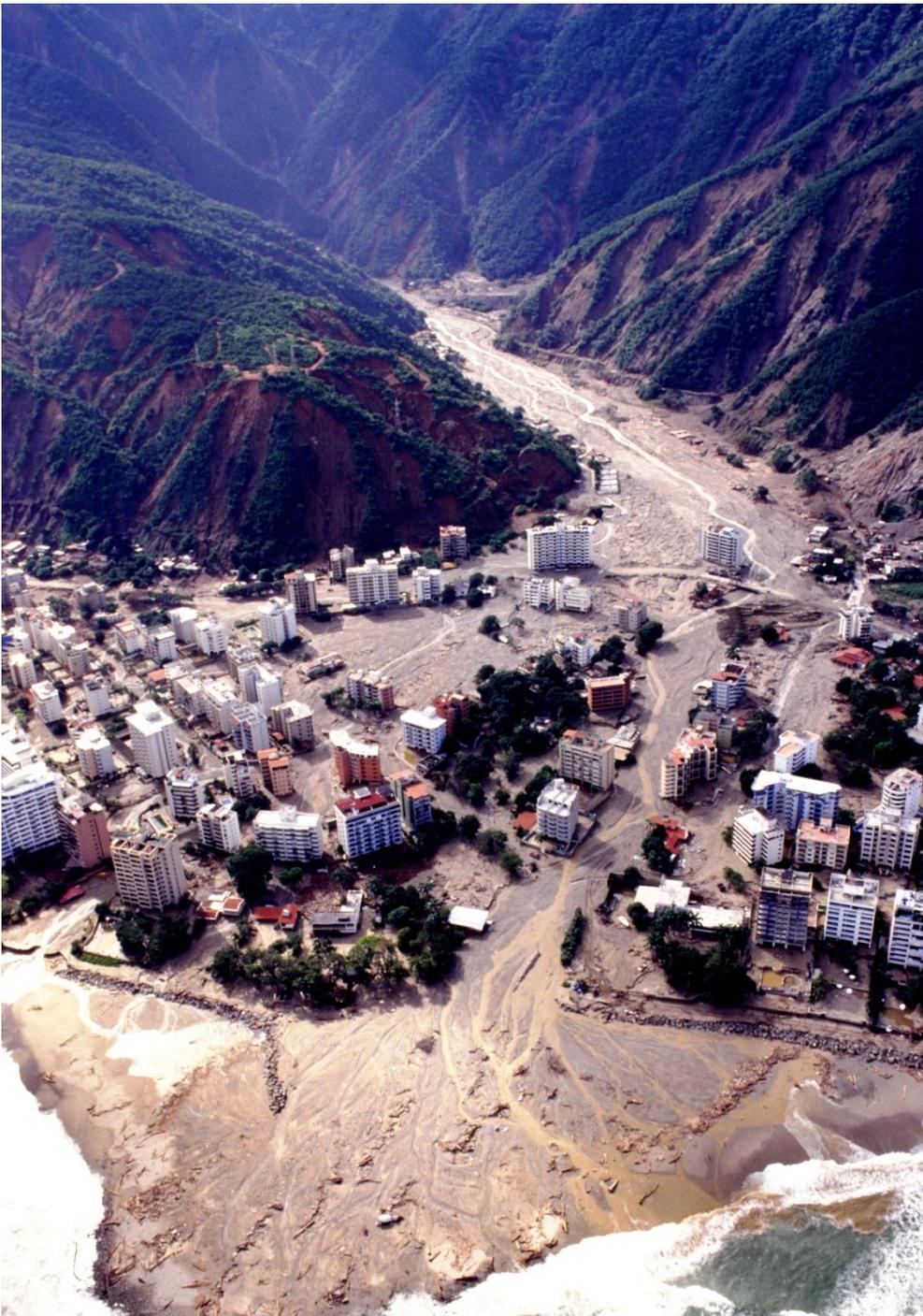
Figure 7. View to south, Vargas, Venezuela, showing numerous landslide scars on steep hillslopes and narrow river channel emanating from Sierra de Ávila mountain front onto highly developed coastal alluvial fan. Note shoreline progradation resulting from massive quantity of sediment delivered onto and across alluvial fan. Photo source: M.C. Larsen, January 2000.
