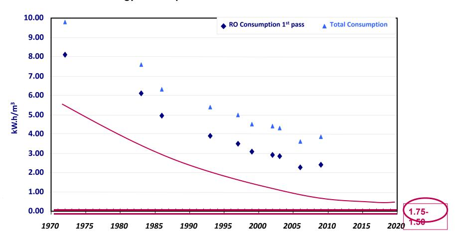
Thermodynamic limit for TDS of 36 g/l at 25°C (conv factor 0.5) : 1.1 kWh/m3
