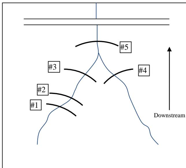
Figure 37. Monitoring silt fences installed in the main drainage, October 2007.
