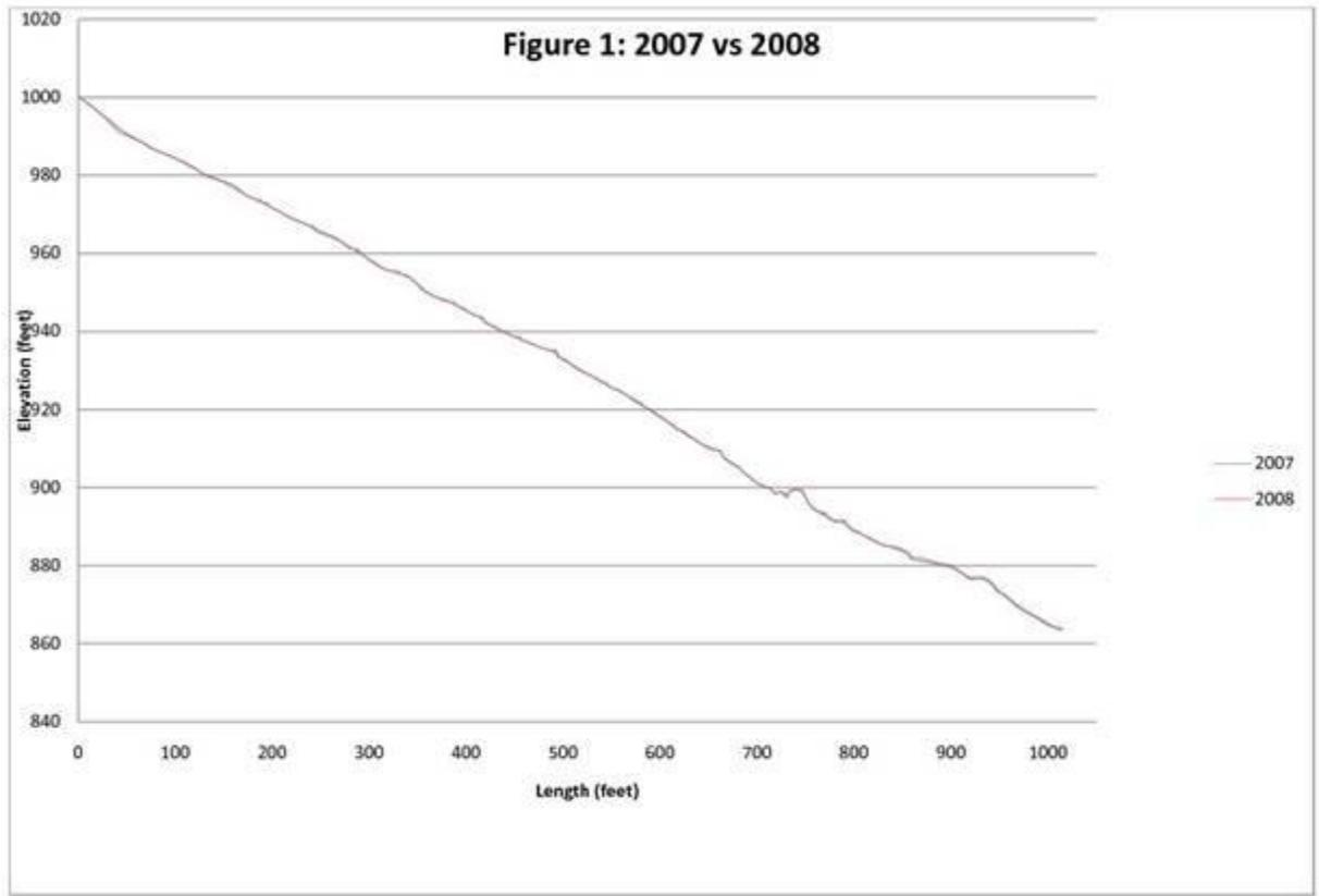
Figure 35. Longitudinal profile of the Mule Deer main channel in 2007 and 2008. Very little change can be seen.
