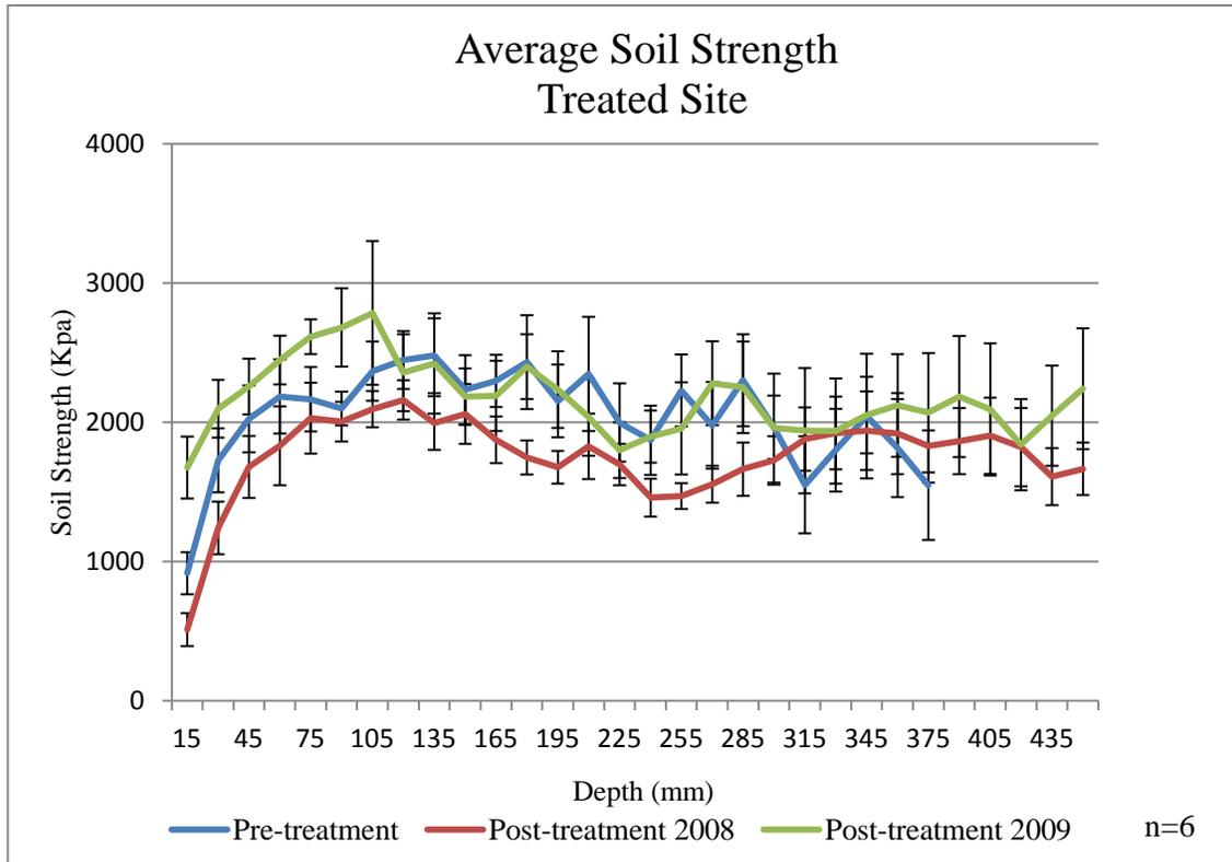
Figure 32. Average soil strength by depth on the treated site.
