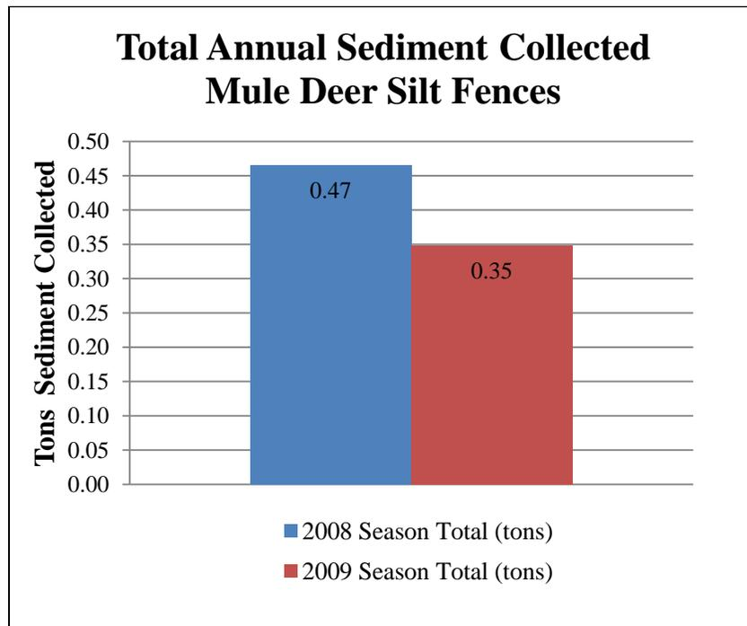
*Figure 39. Graph of sediment collected from silt fences, 2008 and 2009.*
