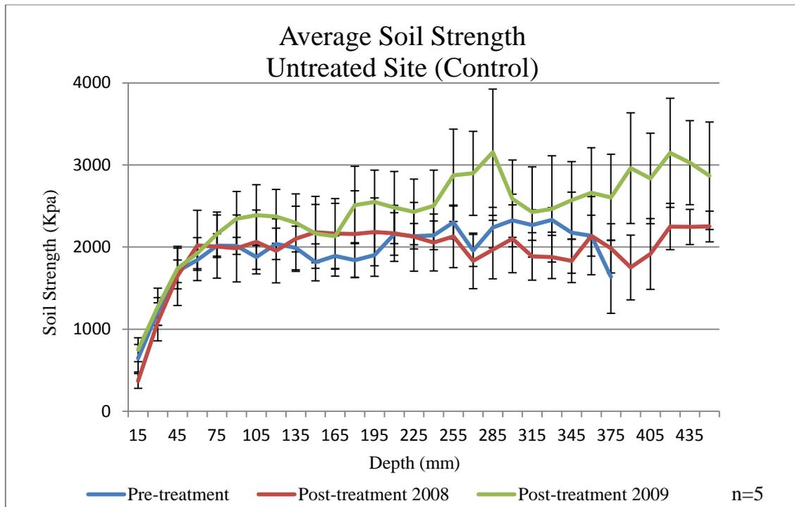
Figure 31. Average soil strength by depth on the untreated site.
