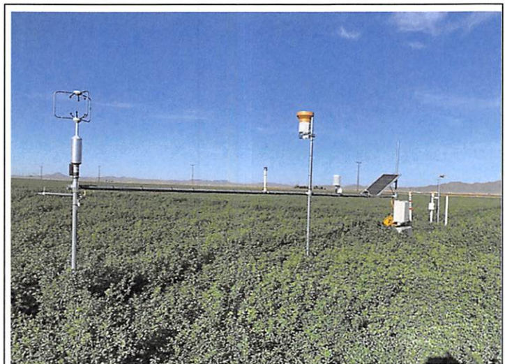
Fig. 2. Fully automated surface renewal and eddy covariance ET station at the field C (Palo Verde).
