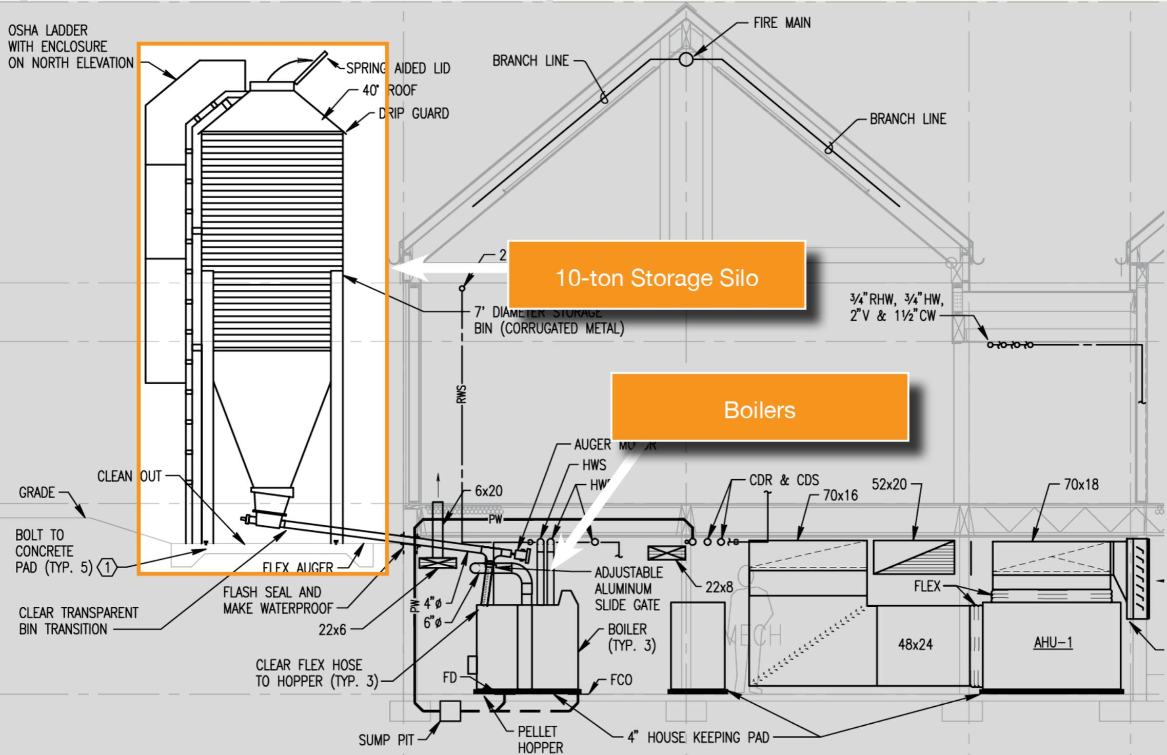
**Storage:** This elevation view shows the proximity of the pellet silo to the pellet boilers in the mechanical equipment room. The silo is 24' tall and 7' in diameter. *Having the mechanical equipment room (MER) on an appropriate exterior wall makes it easy to move the fuel (pellets in this case) from the storage silo or bin to the boiler.*
