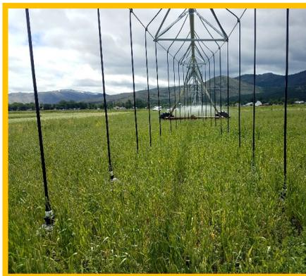
Low elevation sprinkler packages for center pivots are being tested in Sierra Valley for increased irrigation efficiency and reduced pumping cost.
