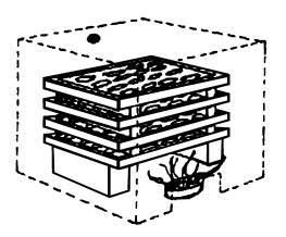
A sulfur box or compartment is necessary. This may be a large cardboard box, provided it is large enough to cover the drying trays and the container for the sulfur. It must be relatively air-tight. A small opening must be provided near the bottom of the compartment for ventilation. Another small opening is necessary near the top of the compartment on the opposite side from the bottom opening.
