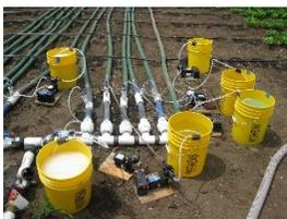
Photo 1. Injection manifold
