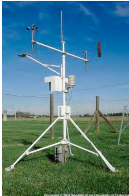
Stations like this measure weather—current conditions like rainfall and windspeed. Climate is the pattern of weather conditions averaged over a very long period of time.
