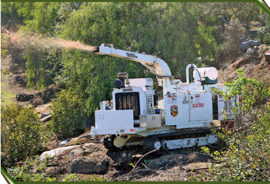
Chippers are an important part of CAL FIRE's fuels reduction work. Both tracked and tow chippers are used where hand thinning projects are being completed.
