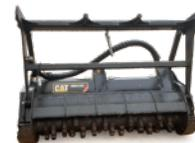
The **masticating attachment** produces a similar result to chipping, except the masticating head does all the work—it can both cut and chip trees up to about four inches in diameter.
