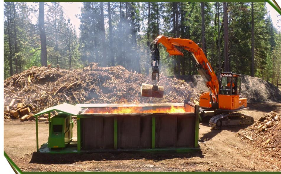
An Air Curtain Burner works by pushing high velocity air over the top of the burn chamber, creating a curtain of air which the rising smoke cannot penetrate. The unburned particulates are pushed back down into the chamber where they reburn until they are light enough to rise through the air curtain.
