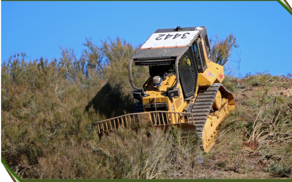
Dozers are used to crush brush by pulling a chain or a ball and chain over the brush. When fitted with a brush rake, dozers are quick and effective at removing and piling brush, preparing it for burning.
