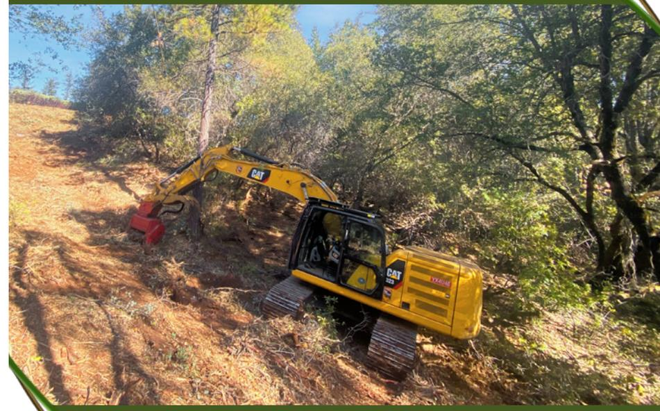
An excavator with a masticator/mulcher attachment can chop or grind vegetation into 1 - 2 inch pieces creating a break in horizontal and vertical fuel continuity. Excavators are an effective tool when creating a shaded fuel break.
