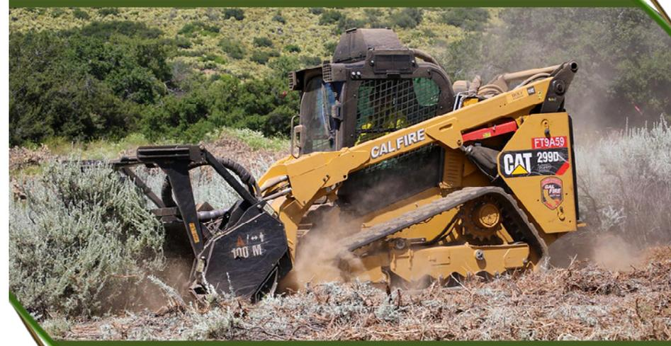
Using the skid steer with attachments, an operator can cut and masticate small and medium sized trees, remove and pile brush, and move piles of cut material to a central location for pile burning or removal.
