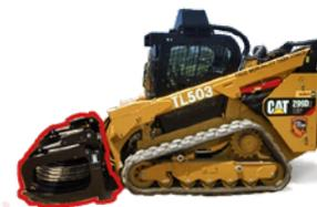
The **brush rake** has a scoop and forks that can be used to clear brush and form piles. It can also clear the ground to bare mineral soil around brush piles, preparing them for burning.
