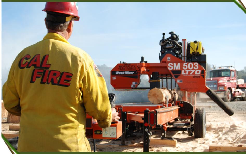
Portable sawmills can be moved and used in the field or at a central location where suitable logs have been staged.
