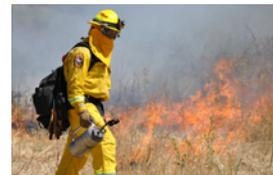
A **drip torch** ignites vegetation by dripping flaming fuel onto the ground.
