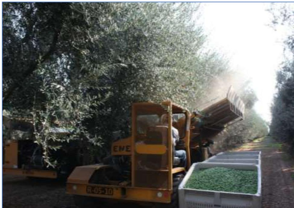
**Figure 3.** Double sided trunk shaking pistachio harvester that can be used in existing orchards, 96 -139 tree per acre, modified with mechanical pruning or hedgerow orchards at higher densities, 180-202 trees per acre.
