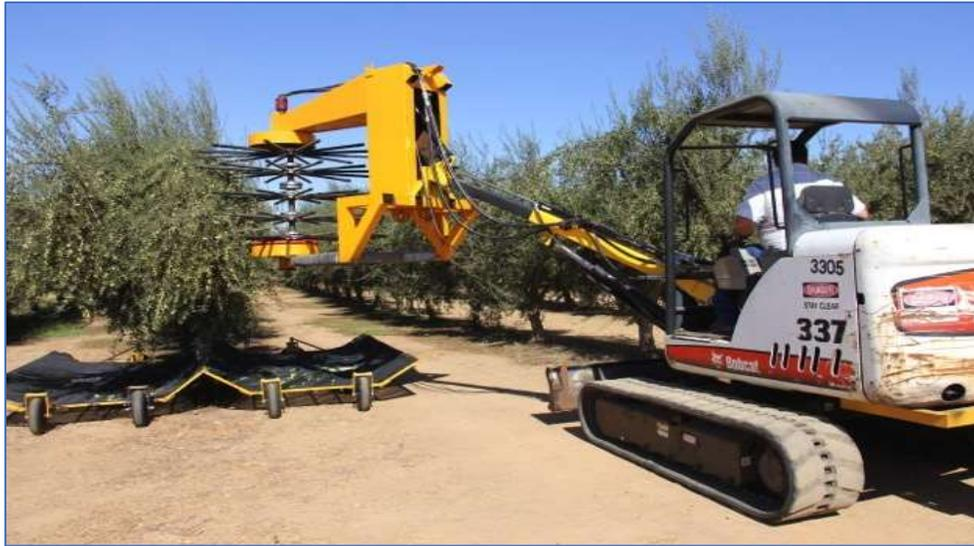
**Figure 2.** A canopy contact harvester adapted from a jatropha harvester. Canopy contact harvesters have higher potential efficiencies with hedgerow orchards that can present a hedgerowed vertical fruiting wall to the harvester head. These orchards can be developed from existing orchards at, 96 -139 tree per acre, with mechanical pruning or developed as a hedgerow at higher densities, 202 trees per acre.
