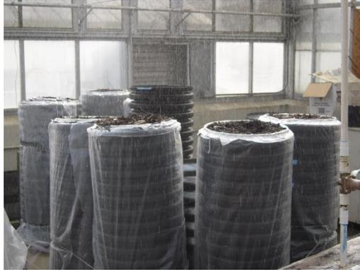
Figure 33. Columns under rainfall simulator.
