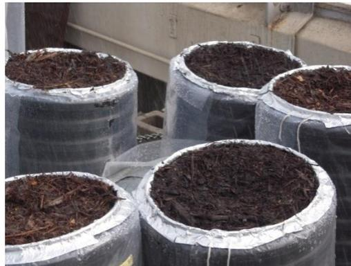
Figure 34. Composting material surface during rainfall experiment.
