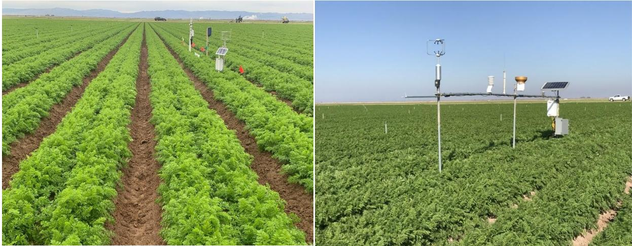
Figure 3. Fully automated ET tower (right) and a multi depths soil moisture sensor monitoring station equipped along with Tule sensor (left).
