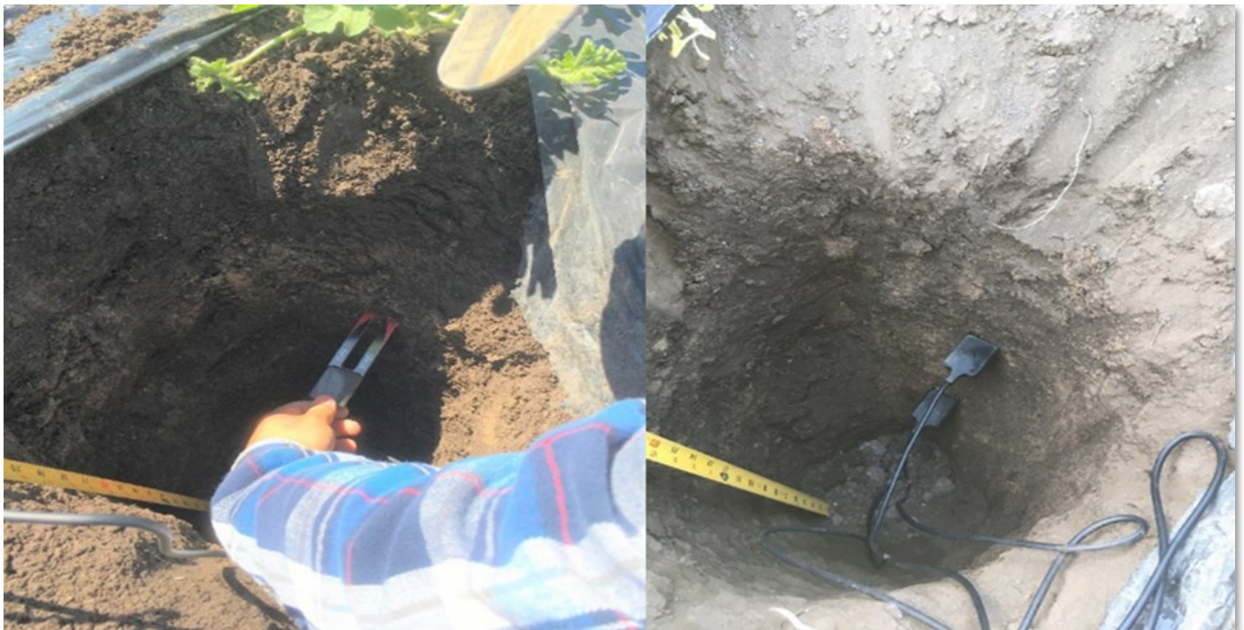
Photo 1. Installation of capacitance soil probe water sensors at a depth of 12, 18, and 24 inches in a clay soil near Stockton, CA.
