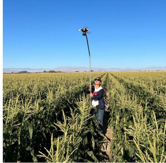
**Fig. 2.** A UCCE research staff is taking canopy infrared images to develop canopy growth curve for the desert sweet corn production systems.
