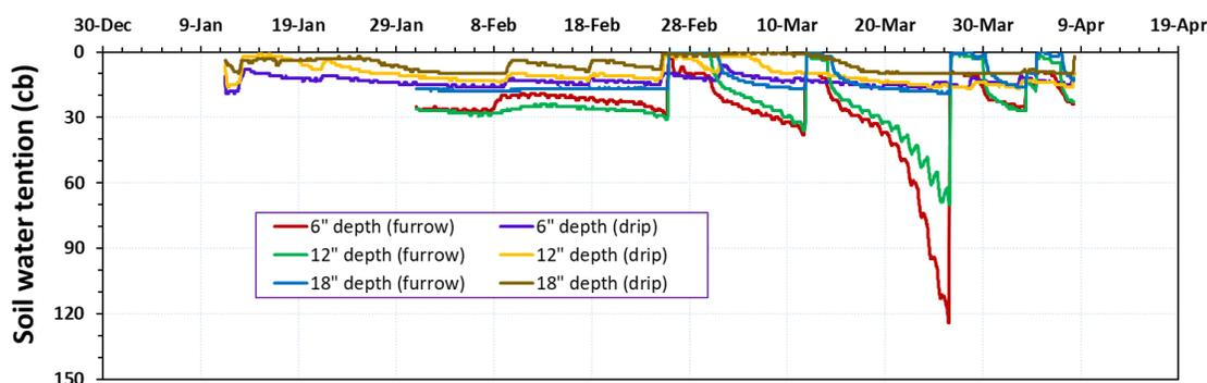
**Fig. 5.** Soil water tension at one drip irrigated sweet corn field against one furrow irrigated sweet corn field over the 2021-2022 season. The data is reported for the depths of 6, 12, and 18 inches for both fields. Maintaining soil water tension at a range of 20-30 centibars (cb) during mid-January through early-April is recommended for most experimental sites.
