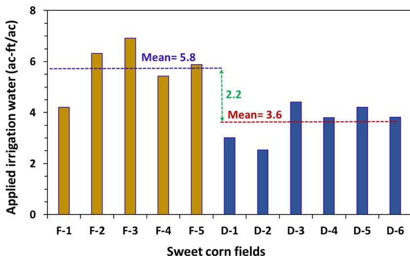
**Fig. 4.** Seasonal applied irrigation water in the furrow irrigated trial fields (F-1 to F-5) and the drip irrigated trial fields (D-1 to D-6). The mean values of seasonal applied irrigation water in each group of furrow and drip irrigated fields are also demonstrated.
