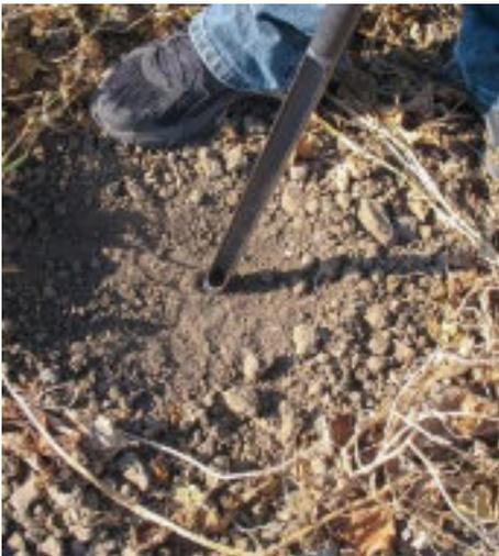
*Taking a soil sample with an auger. Note that organic debris on the surface has been moved aside prior to taking the sample. Photo by Dr. Daniel J. Geisseler. © The Regents of the University of California.*
