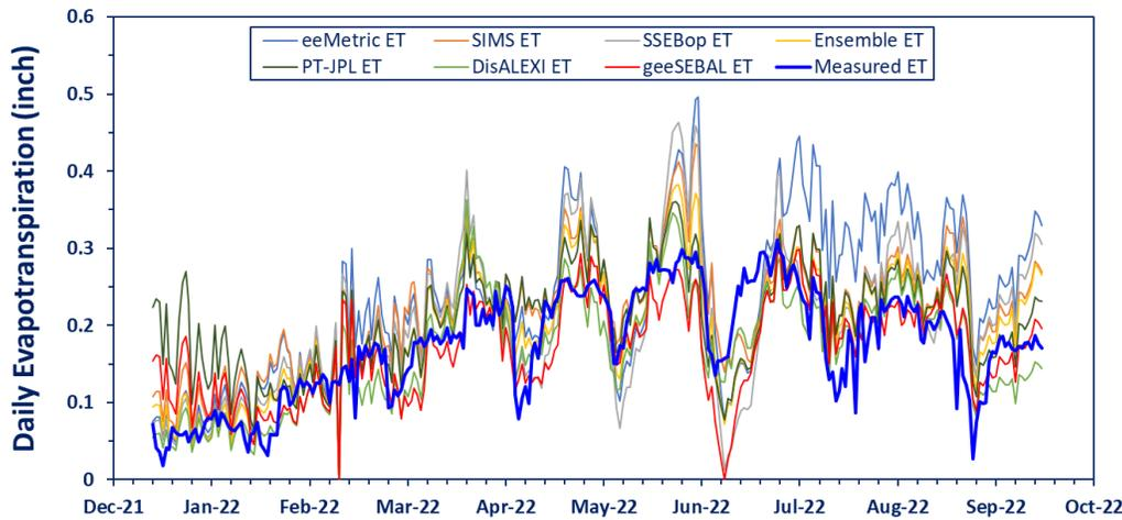
Fig. 4. Daily evapotranspiration estimated by the OpenET models and measured using surface renewal equipment in an alfalfa field nearby Holtville, California. The alfalfa field was harvest eight times during the study period (January 1<sup>st</sup>, 2022, through September 30<sup>th</sup>, 2022).
