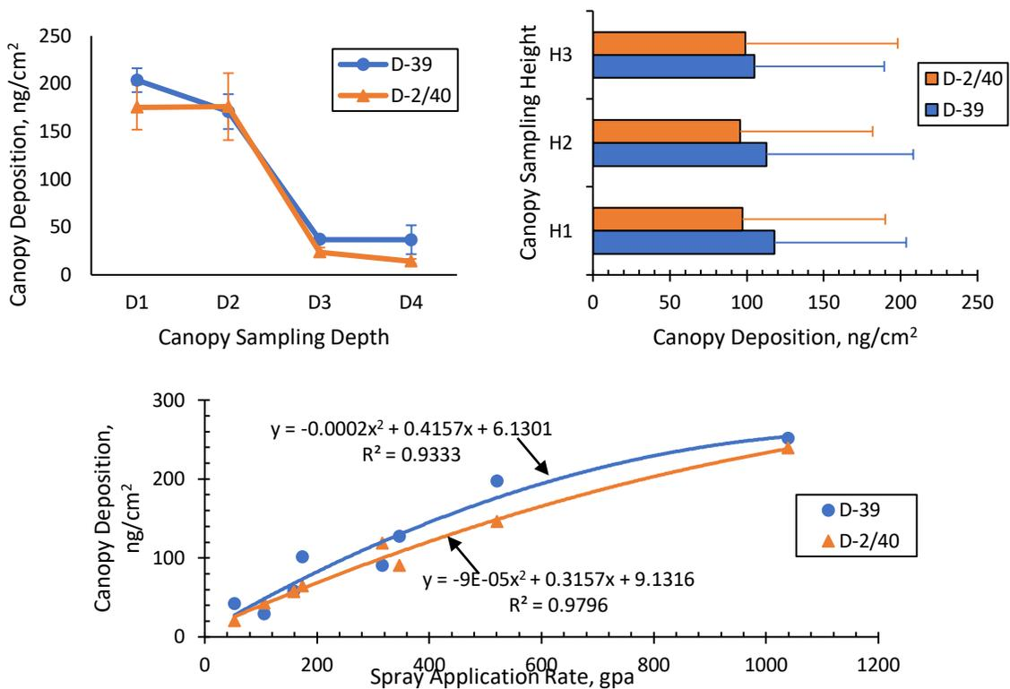
**Figure 3.** Mean canopy deposition for all spray treatments with respect to: a) sampling depth; b) sampling height; and c) application rate.
