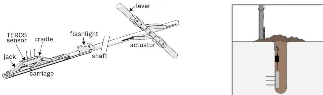
Figure 3 (left) Teros Borehole Installation tool and figure 4 (right) proper Teros 11 sensor placement
