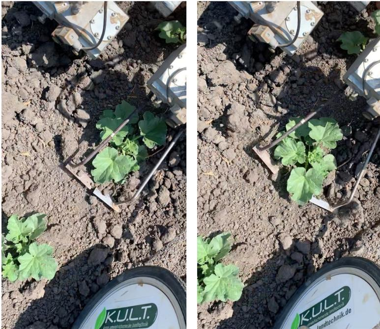
**Figure 2. Robovator blades are closed (left) between plants, then open at a present “buffer zone” when a plant is detected by the onboard cameras.**
