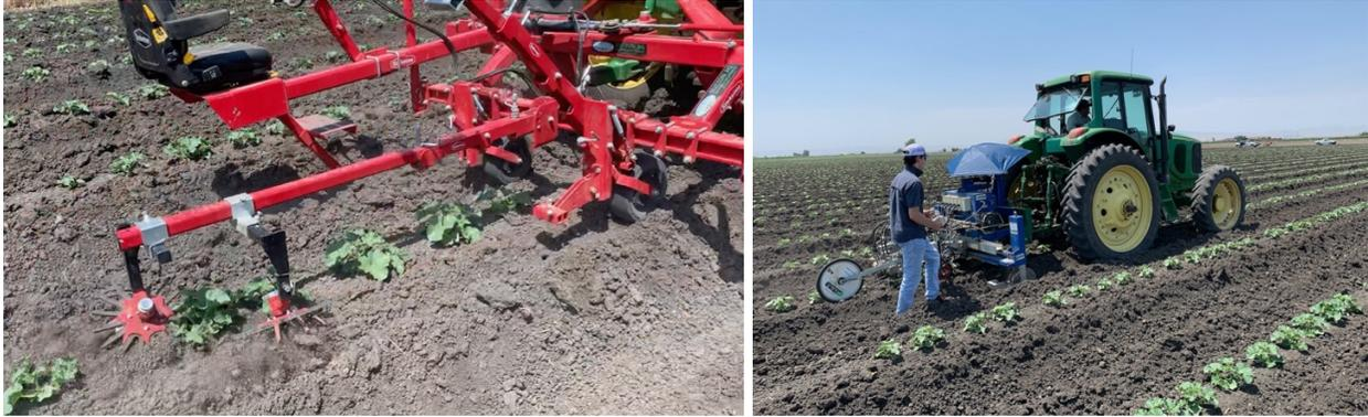
**Figure 1. Finger weeder (left) and Robovator cultivation at 3 weeks after seeding.**
