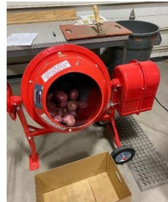
**Figure 2. Cement mixer setup for evaluating tuber skinning.**
